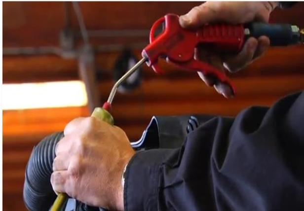
6. Use air blower with rubber tip. Hold steel tube firmly into head, blow compressed air into steel tube. A popping noise may be heard from carbon plug in passages blowing out.
